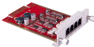
Module 2FXOS (2 Ports FXO & 2 ports FXS)
